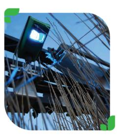
Natural NIR is everywhere in the environment and therefore WEEDit must run constant calibrations measuring the level of background NIR, this is all done automatically and without you knowing it.
